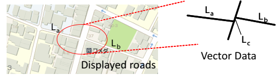
Figure 11: Intersection having slight misalignment.
